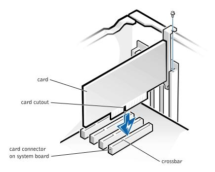
Make sure that the card is fully seated and that its bracket is within the card slot.
